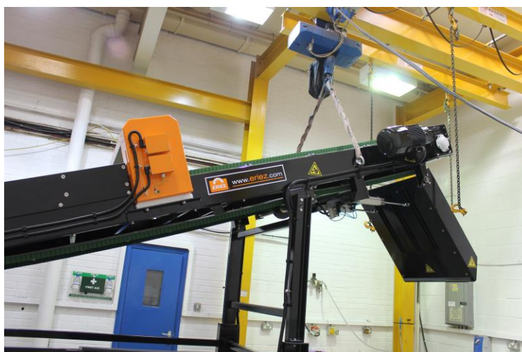
Pneumatic Reject System on the E-Z Tec 9000 R Metal Detector
