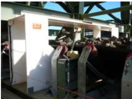
Quarry application of industrial metal detector MA 3500 Bridge Coil
