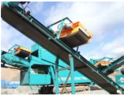
CP overband magnets on mobile crushers and conveyors.
